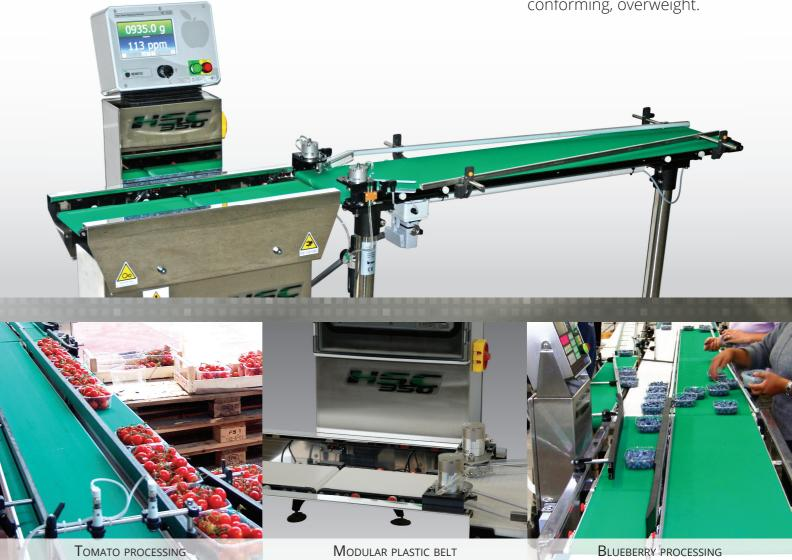
The "Flipper" sorting system can work with delicate packages, even open ones, without the risk of damaging or spilling the product.
